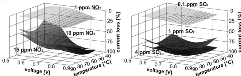
Figure 1: Current loss depending on voltage, temperature and concentration of contaminant (left: NO<sub>2</sub>; right: SO<sub>2</sub>)
